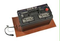
Battery heater not recommended for nickel cadmium batteries. When batteries are placed in an insulated battery box, a thermostat is recommended to sense battery box temperature to prevent overheating the battery.
